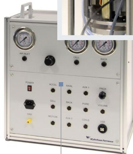
**Compact Control Panel** connects to the PC and includes all control, power supply and pneumatic devices. This system also includes air actuators (I/P converters) and all necessary amplification equipment.
