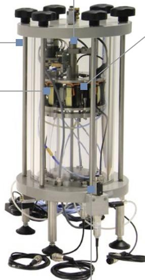
**Pressure transducers** for the measurement of cell, pore and back pressure.
