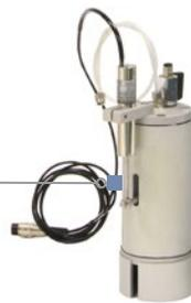
**High-sensitivity volume change device** with high-precision LVDT transducer.
